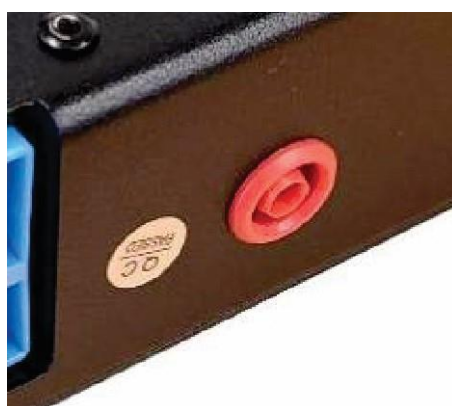
Figure 12: Ignition Trigger Input
